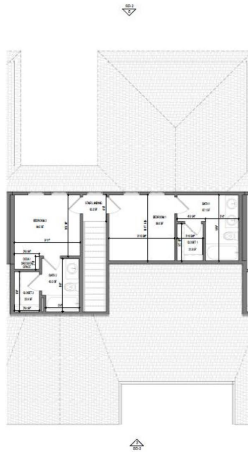
2 SECOND FLOOR PLAN - BROWNSTONE TH SCALE: 1/4" = 1'-0"
